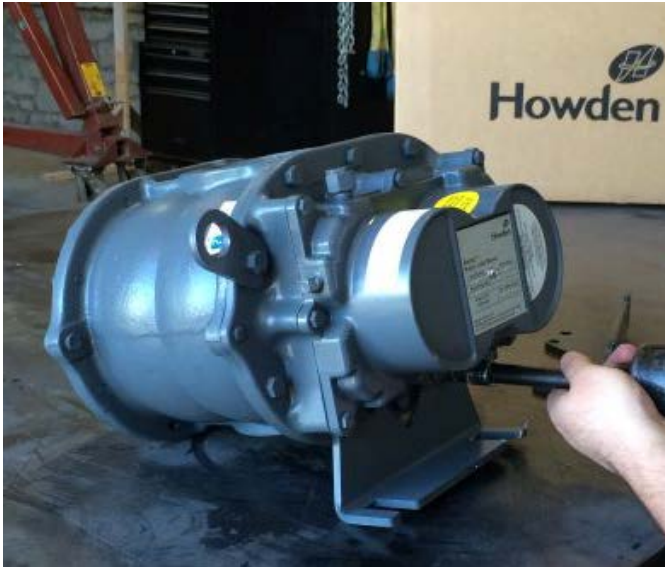
Step 2. Remove the lifting tab and bolt from the non-shaft side.
