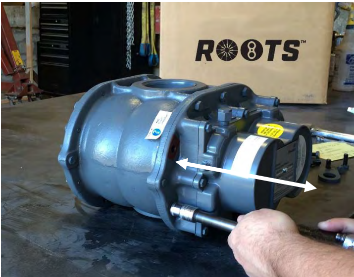
Step 3. Install the feet for the new configuration. Hand tighten the bolts at this time.
