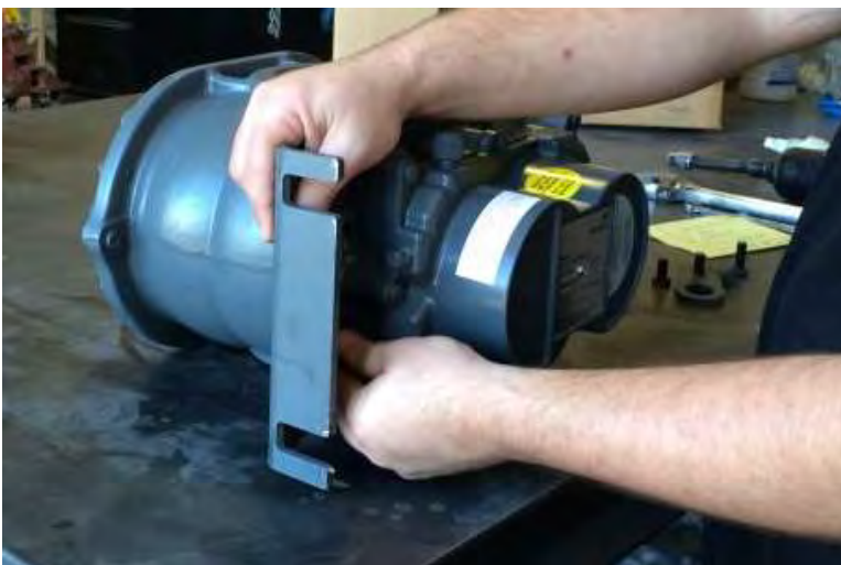
Step 3. Install the feet for the new configuration. Hand tighten the bolts at this time.
