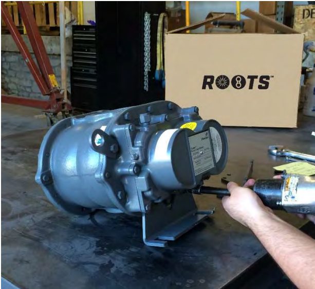
Step 2. Remove the lifting tab and bolt from the non-shaft side.
